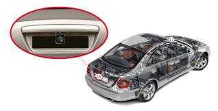
7. To set up the rear-view camera so that it automatically triggers the rear-view camera display once reverse gear is selected, connect the red wire to the positive wire of your vehicle's reverse lights (see illustration). Seek expert advice before attempting this installation. To access the reverse light wires we advise you refer to the car manual for further instructions related to your vehicle.
